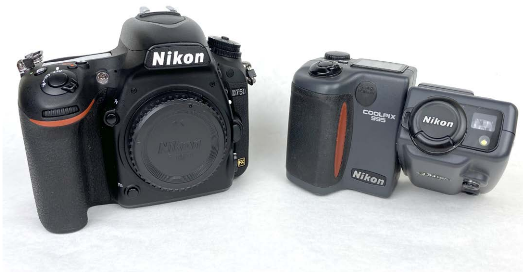
Figure 2. A current model DSLR camera body on the left (Nikon D750) and a vintage point and shoot camera (Nikon 995) from 2001. The 995, with its 3.34 megapixel sensor and excellent macro imaging firmware, was popular for numismatic photography a couple of decades ago.
