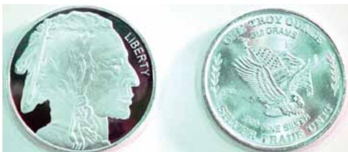
SG testing was done on both pieces. It was clear the Buffalo round was not pure silver just based on its "dry weight" alone. However, the SG testing gave some insight into what its composition might be. Below is a table with the results of the SG testing.
