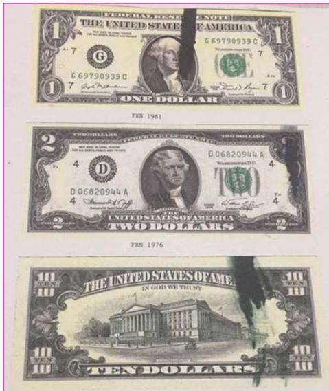
Ink smear errors occur from inadequate cleaning of the printing press. The amount of residual left on the surface of the plate determines the size and shape of the smear. Samples pictured are considered moderate smear grade.
